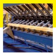
Brookstech Laminated Timber Products are a factory-produced, 'engineered' material made by gluing together and clamping accurately machined, defect-free lamellas of solid timber.
